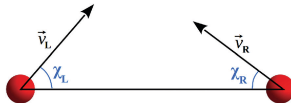
Fig. 7 Schematic representation of vector parts of HOs, forming a (strained) bond between the left-end (L) and right-end (R) atoms of this bond.
