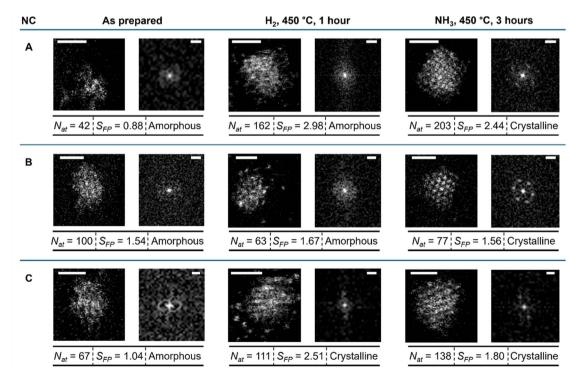
Fig. 4 Evolution of Ru/GNF after H2 treatment for 1 hour and NH3 decomposition reaction for 3 hours: identical location observation of individual nanocluster. STEM images with FFT patterns shown on the right side, and key nanocluster parameters below each image. The scale bar in the STEM image is 1 nm. The scale bar in FFT patterns is 5 nm $^{-1}$ .
