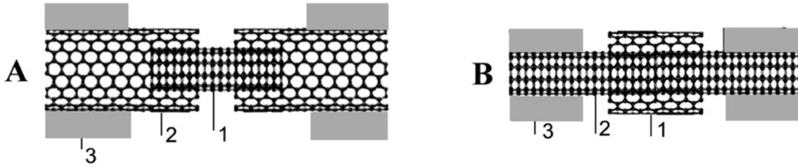
**Fig. 1** Schematics of an electromechanical nanothermometer based on DWNT: A) a shuttle nanothermometer with the movable inner wall, B) a telescopic nanothermometer with the movable outer wall. 1 is the movable wall, 2 is the fixed wall with the attached electrodes 3.
